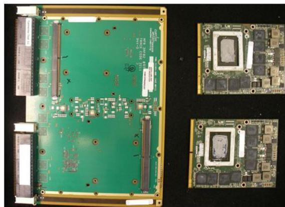
Figure 1. Photo of disassembled vibration test vehicle (MXM heat sinks and other metalwork removed)
