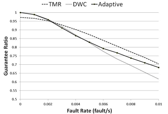
Fig. 3. Effect of Fault Rate on Task Rejection ( $N_{PRRs} = 12$ ,  $t_{exec} \in [10, 100]$ ,  $t_{deadline} \in [100, 200]$ ,  $\lambda_{arrival} = 0.075$ )
