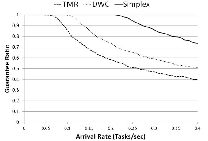
Fig. 2. Effect of Arrival Rate on Fault-Free Operation ( $N_{PRRs} = 12$ ,  $t_{exec} \in [10, 100]$ ,  $t_{deadline} \in [100, 200]$ )
