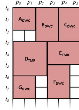
Fig. 5. Resource Fragmentation from Adaptive Placement
