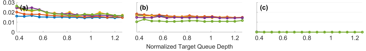
Fig. 9: Normalized Packet Retransmission at 70% of link bandwidth for 8-to-1 incast streaming PUT workload
