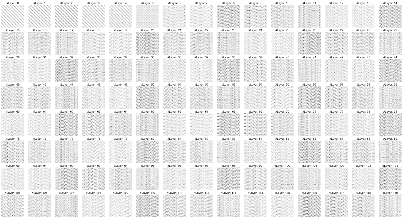
Fig. 1: Pattern of SpDNN weights for 1024 neurons on 120 layers (each 1024 \times 1024 matrix has 32768 nonzeros, 97% sparsity).
