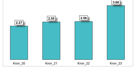
Fig. 4. Speed-up for parallel Bellman Ford implementation with respect to serial Bellman Ford on Kronecker graphs.
