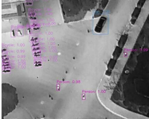
Fig. 5: Sample Training Image from ThermalUAV Dataset showing small targets (person, bicycle) and large targets (car) in a single image.
