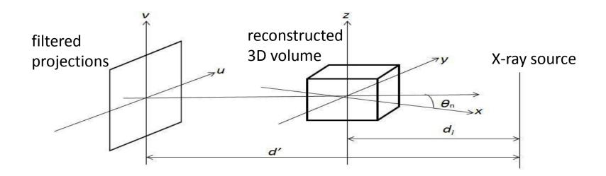
Weighted Projection: Weighted and ramp filtered raw data produce filtered projections Q<sub>1</sub>, Q<sub>2</sub>, ..., Q<sub>k</sub>, collected at an angle ∂n where 1 ≤ n ≤ K.
