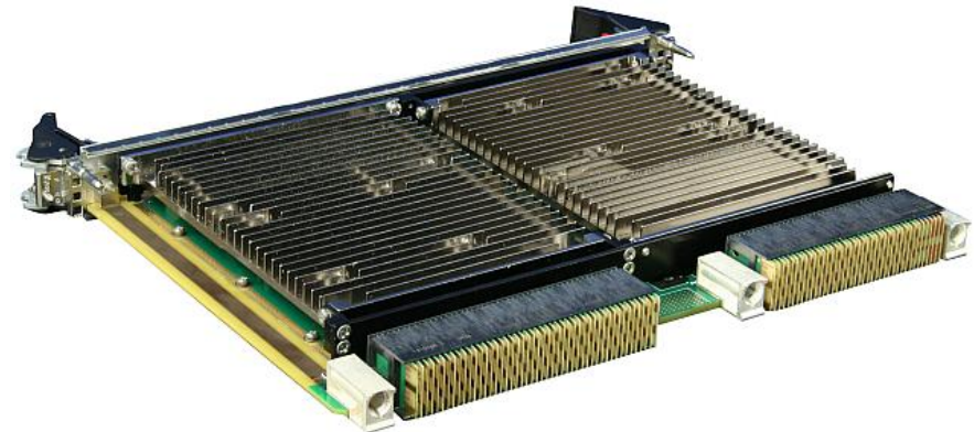
6U air cooled module with 2 MXMs
