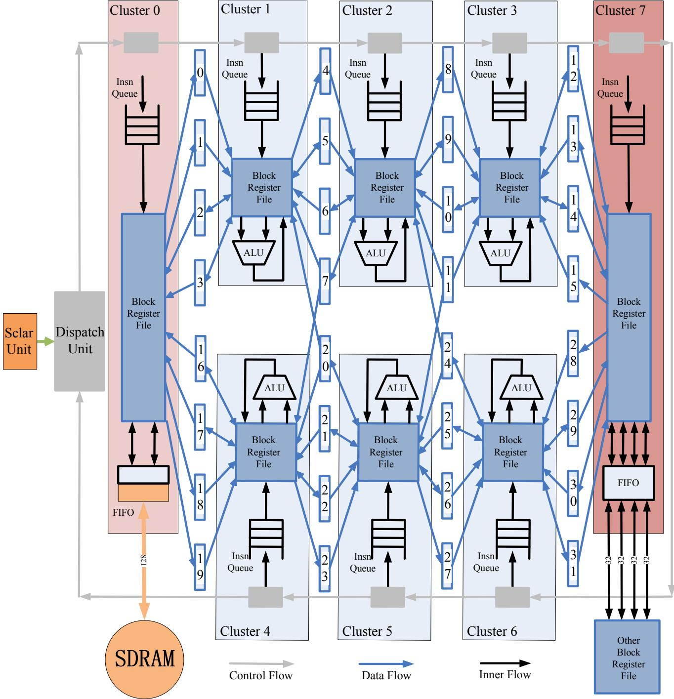
Fig.2. The proposed vector unit contains one dispatch unit and 8 clusters, which has 1 load/store unit (cluster 0), 6 compute units (clusters 1-6) and 1 external unit (cluster 7). The cluster 1 reads from block registers 0,1,2,3,5,6,7, and 20, writes to block registers 2,3,4, and 5.
