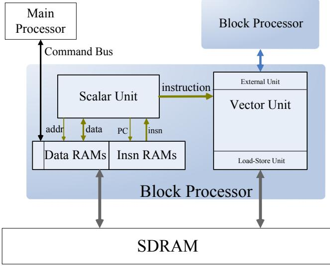
Fig.1. The block diagram of Block Processor. Block Processor consists of the scalar unit and vector unit.
