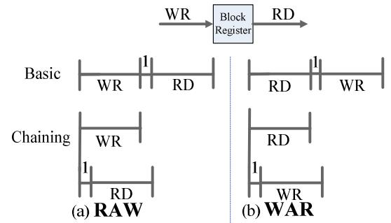
Fig.3. Timings between write port and read port of the block register, both basic and chaining. The 1-clock cycle delay is the latency of crossover between read and write operations.
