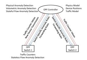
Fig. 1. L-IDS Controller and Switch Roles
