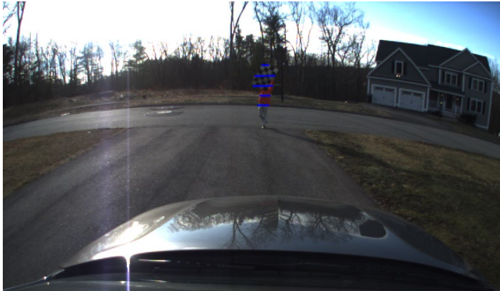
LiDAR-camera projection validation on single camera frame
