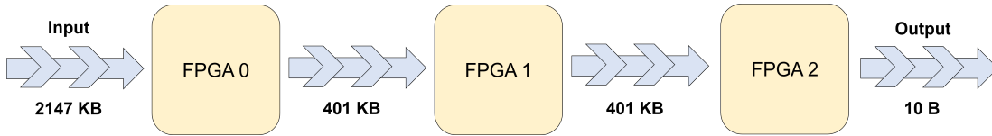
Fig. 2. Sizes of the data transfers for one inference of the multi-FPGA ResNet-50 accelerator
